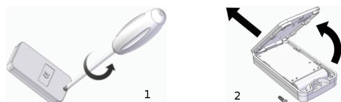
**EN** Unscrew the screw on the back of the remote control, lift the cover, remove the battery and replace it with the new one, paying attention to the polarity. Close the cover and fasten it with the screw.
